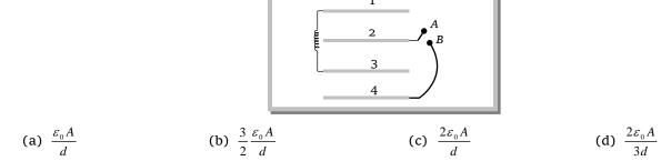
**262.** Consider the situation shown in the figure. The capacitor A has a charge q on it whereas B is uncharged. The charged appearing on the capacitor B a long time after the switch is closed is
